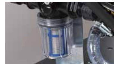
Readily serviceable external suction filter
